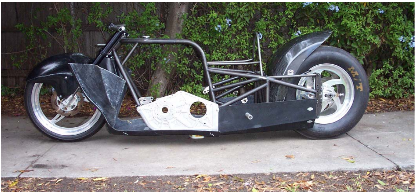
The Parker Racing Pro Stock Motorcycle with body and engine removed.
