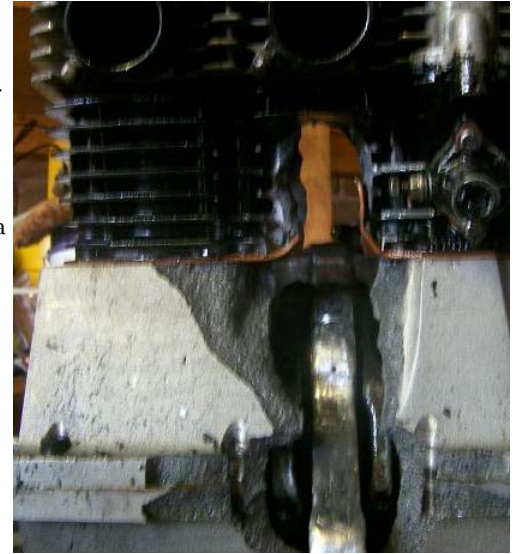
The damage inflicted on Phil's motor. Your not normally meant to be able to see straight through that part of the motor!!!
