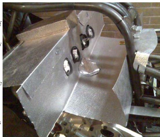
A new air box being constructed on the Parker Racing Pro Stock Hayabusa.
