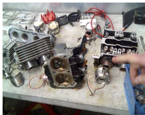
Some dead engine parts after a nitro explosion. Yes that is a cylinder head in half!!!
